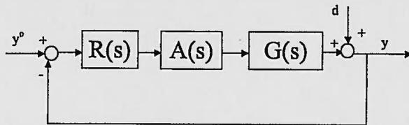
NO, SONO LE STESSA PERCHÉ  $A(s)$  INTRODUCE SOLO UN POLO  $p = -\frac{1}{0,002} \gg \omega_c = 1$  E QUINDI NON ALTERA LE CARATTERISTICHE DI  $L(s)$  RILEVANTI PER LE PRESTAZIONI AL PUNTO 2.1
