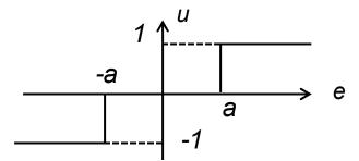
Set  $y^{\circ}(t)=0$ ,  $t \ge 0$ , and determine how parameter a should be set so that the describing function method predicts some limit cycle.
